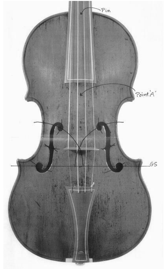
Figure 9 - A. Amati 1564 showing placement of f-holes
