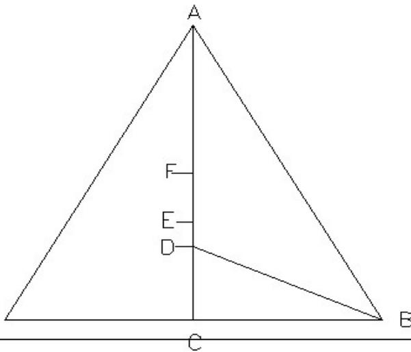
Figure 1 – The Proportioning Triangle: The distance AB is one-third the pin length. BC is one-half the length of the side; therefore, one-half AB. The line AC is perpendicular to the side opposite point A. CD is one-fourth AC. CE is one-third AC. CF is one-half AC. BD is the hypotenuse of the right triangle BCD.
